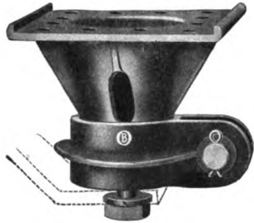
Fig. 629—Exterior View of Drawbar Anchorage
