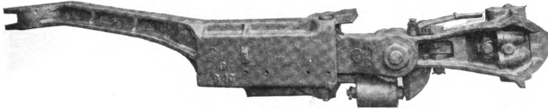
Fig. 600—High Capacity Draft Gear Housed in Swinging Pocket with Westinghouse Automatic Coupler as Applied to Interborough Subway Cars Forsyth Bros. Company
