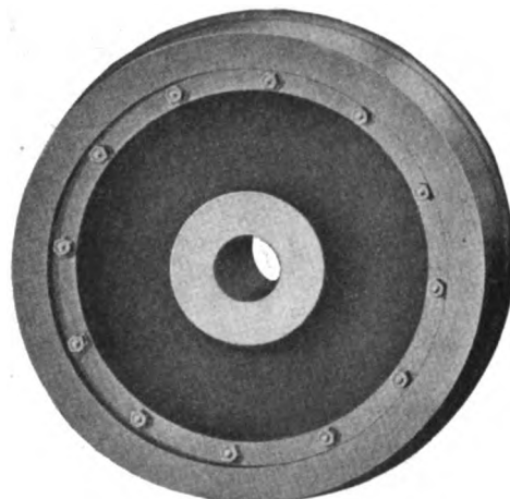
Figs. 1643-1644—Steel Tired Wheel with Double Plate Cast Iron Center, Tire Held by Bolted Fastening Railway Steel-Spring Company
