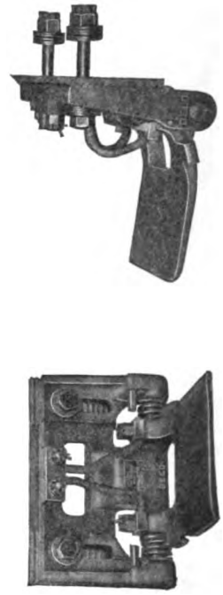
Figs. 1857-1858—Slipper Type Third-Rail Shoe for Underrunning Third Rail; Capacity, 800 Amperes General Electric Company
