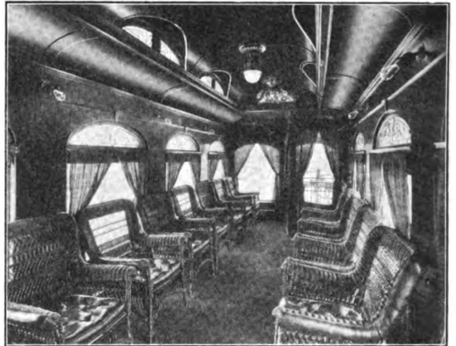
Fig. 166—Interior of Observation Compartment of Private Car Shown in Fig. 167 Niles Car & Manufacturing Company, Builder
