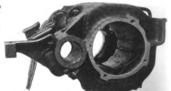
Fig. 1667—Westinghouse, No. 310, Box Frame, Interpole, Direct-Current Motor, with Armature Removed
