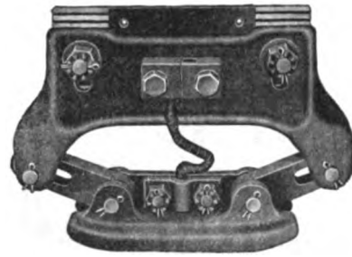
Fig. 1861—Gravity Type Third-Rail Shoe for Overrunning Third Rail General Electric Company
