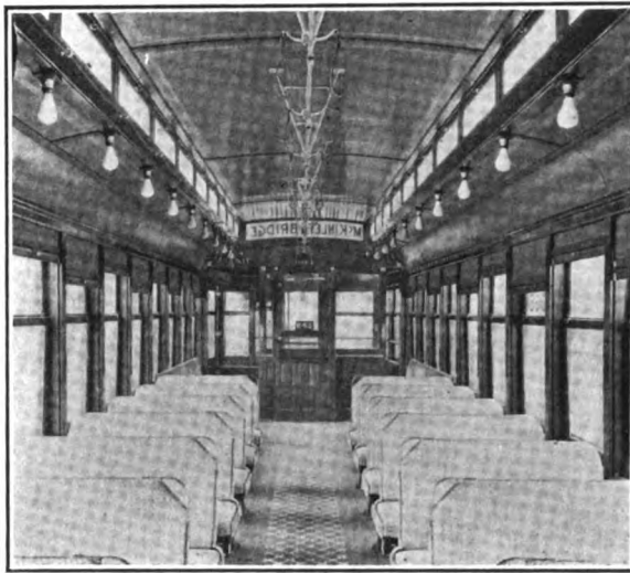
Fig. 49—Interior of Double-Truck, Single-End, Closed, Pay-as-You-Enter Car; Illinois Traction System The J. G. Brill Company, Builder
