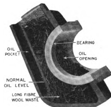
Cross section of waste - packed, Axle Cap and Bearing for Box-Frame Motor.
