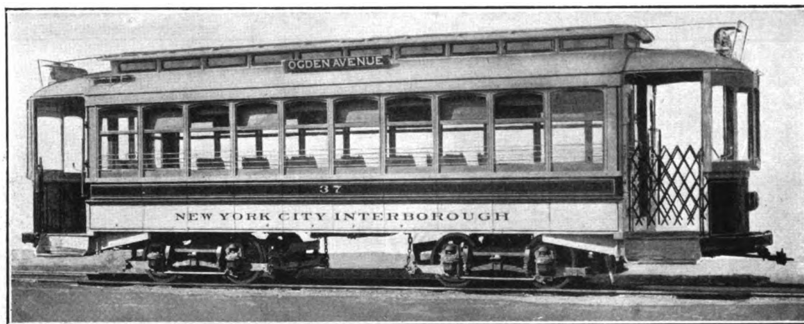
Fig. 76—Double-Truck, Double-End, Semi-Convertible Car with Portable Vestibules The J. G. Brill Company, Builder
