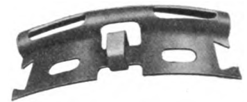
Fig. 1495—Steel Back Reinforcement for Flanged Brake Shoes
