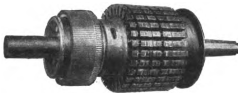
Fig. 1697—Armature Core and Commutator Mounted on Shaft
