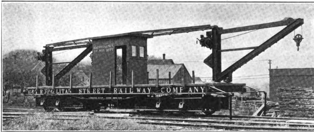
Fig. 236—Double-Track Crane Car with Motor-Driven Cranes at Each End Metropolitan Street Railway, New York
