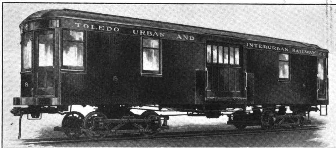
Fig. 193—Freight and Express Trail Car with Arch Roof Niles Car & Manufacturing Company, Builder
