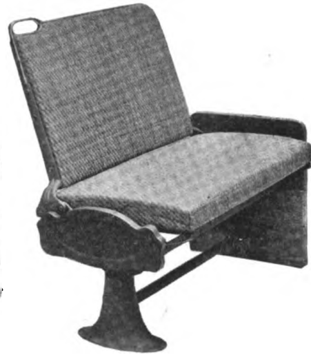
Fig. 1261—Universal Car Seat, Wheeler Reversing Type; Pressed Steel Pedestal, Single Foot Rest, No. 327SC
