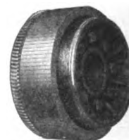
Fig. 1695—Bolted Type Commutator, Front View
