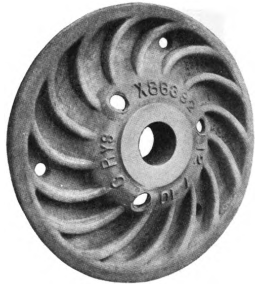
Fig. 1604—Back of Double Plate "F. C. S." Cast Iron Wheel Griffin Wheel Company
