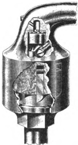
Fig. 570—Sectional View of Gravity Ratchet Brake Handle A. & W. Co.
