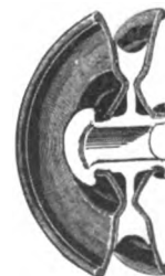
Fig. 1913—Section of Lumen Bronze Trolley Wheel
