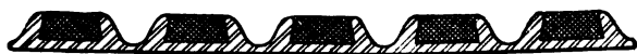
Fig. 927—Section Through American Mason Safety Step Tread American Mason Safety Tread Company
