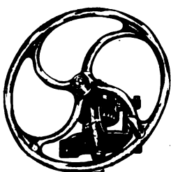
Fig. 570—Sectional View of Gravity Ratchet Brake Handle A. & W. Co.
