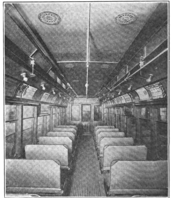
Fig. 1359—Interior View of Car Showing Exhaust Registers in Ceiling
