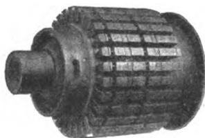
Fig. 1693—Armature Core on Spider
