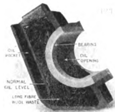
Fig. 1673—Axle Cap and Oil Well for Box Frame Motor
