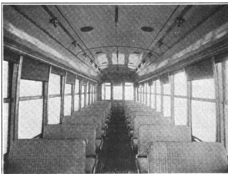
Fig. 77—Interior of Arch-Roof, Semi-Convertible Car Shown in Fig. 78 The J. G. Brill Company, Builder
