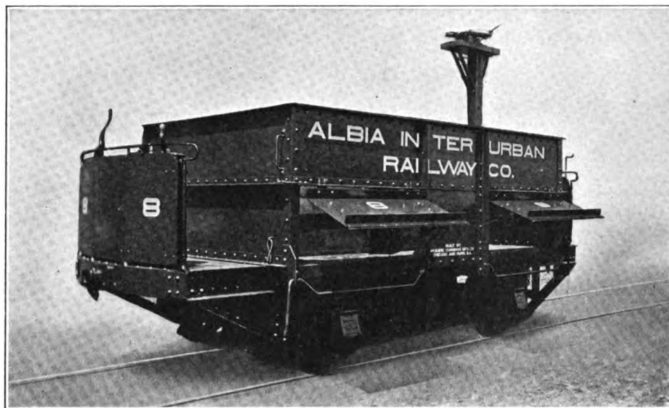
Fig. 233—Single-Truck, All-Steel, Motor Coal Car with Drop Sides McGuire-Cummings Manufacturing Company, Builder
