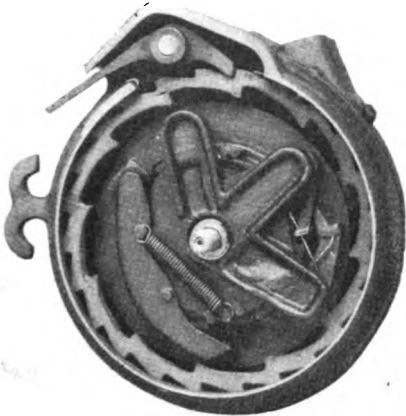
Fig. 1328—Interior of Earll Trolley Retriever, No. 5
