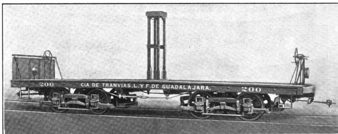
Fig. 228—Motor Flat Car with Center Trolley Stand The J. G. Brill Company, Builder
