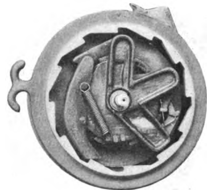
Fig. 1327—Interior of Earll Trolley Retriever, No. 4
