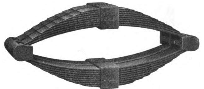
Fig. 1573—Double Full-Elliptic Spring, Sectional Type
