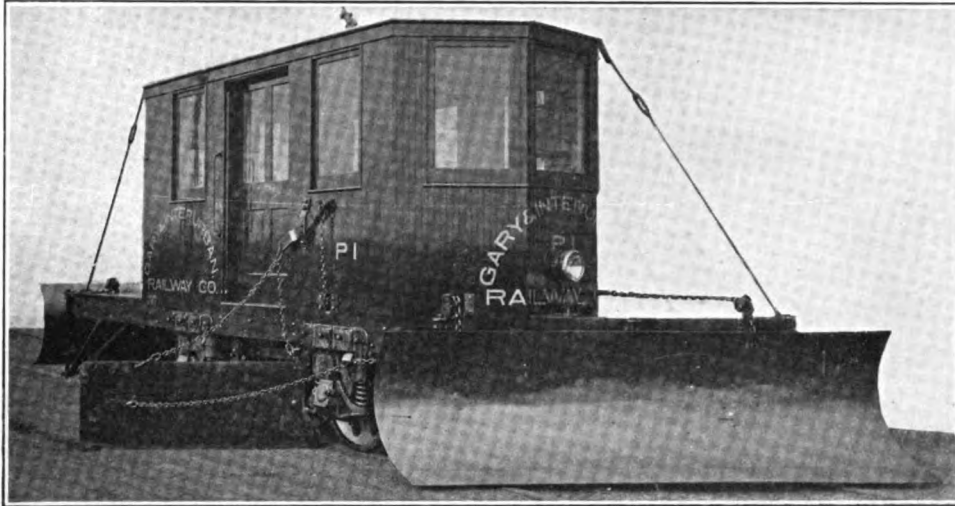
Fig. 219—Single-Truck, Double-End, Shear Plow McGuire-Cummings Manufacturing Company, Builder
