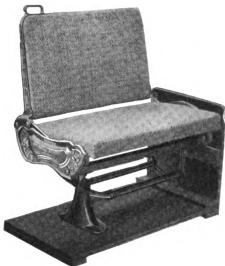
Fig. 1297—Winner Car Seat, with Shifting Cushion and Double Foot Rest
