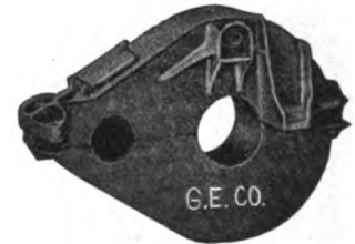
Fig. 1539—Malleable Iron Gear Case General Electric Co.
