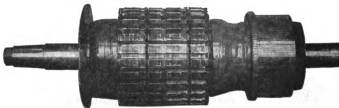
Fig. 1699—Armature and Insulation in Place Ready for Winding
